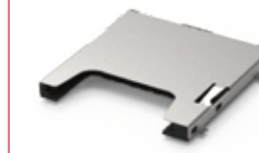
104I-TA01 SD 4.0 Socket, UHS-II, Top Mount, Push-Push Type, w/switch/card lock
