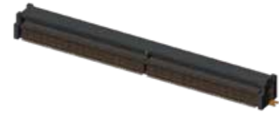
125B-78C00 MXM 3.0 Connector, 314 pin, H=7.8mm, Pitch=0.5mm, 5u"
