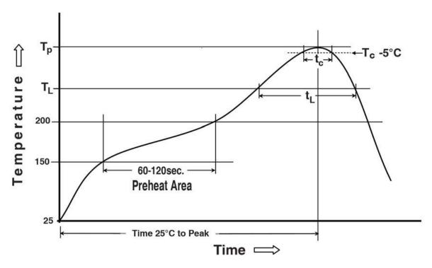
Preheating temperature:  $150 \sim 200$ °C,  $60 \sim 120$  seconds Liquidus temperature (TL): 217°C,  $60 \sim 150$  seconds
