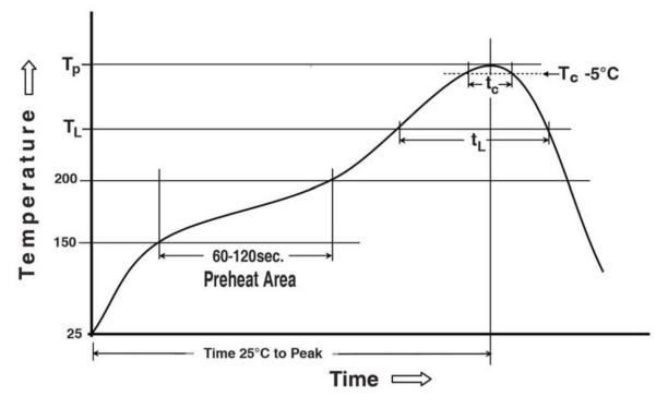
Preheating temperature: 150 ~ 200°C, 60~180 seconds Liquidus temperature (TL): 217°C, 60~150 seconds Peak temperature: 260°C Time within 5 °C of peak temperature (Tc): 255°C, 30seconds
