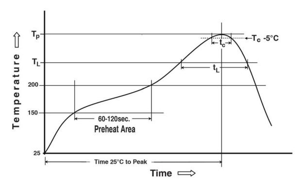
Preheating temperature: 150  $\sim$  200°C, 60 $\sim$ 180 seconds Liquidus temperature (TL): 217°C, 60 $\sim$ 150 seconds
