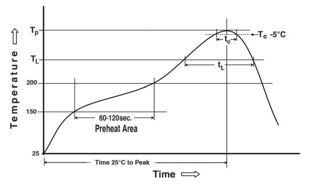
Preheating temperature: 150 ~ 200°C, 60~120 seconds Liquidus temperature (TL): 217°C, 60~150 seconds Peak temperature: 260°C Time within 5 °C of peak temperature (Tc): 255°C, 30seconds
