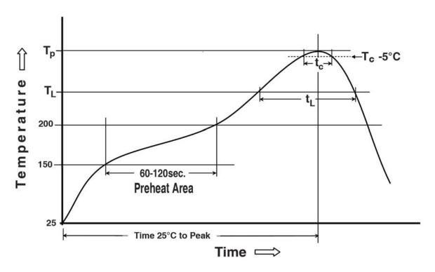
Preheating temperature: 150 ~ 200°C, 60~120 seconds Liquidus temperature (TL): 217°C, 60~150 seconds
