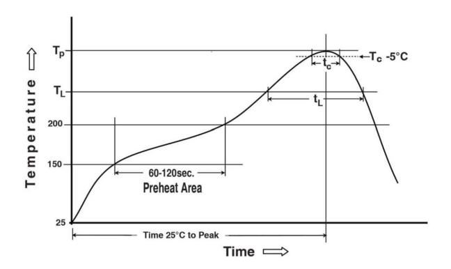
Preheating temperature:  $150 \sim 200^{\circ}$ C,  $60 \sim 120$  seconds Liquidus temperature (TL):  $217^{\circ}$ C,  $60 \sim 150$  seconds
