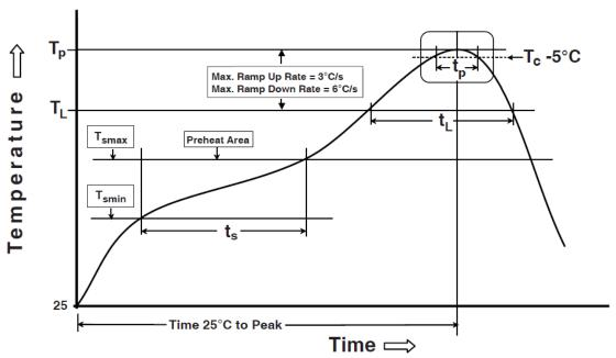
Preheating temperature:  $150 \sim 180^{\circ}\text{C}$ ,  $90\pm30$  seconds Liquidus temperature (TL):  $230^{\circ}\text{C}$ ,  $30\pm10$  seconds
