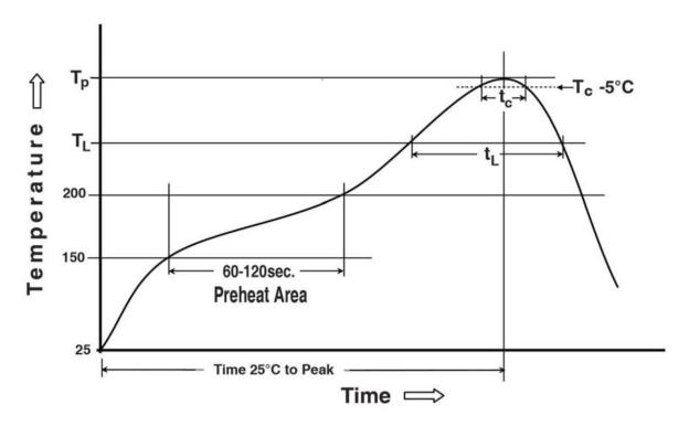
Preheating temperature:  $150 \sim 200^{\circ}\text{C}$ ,  $60 \sim 120$  seconds Liquidus temperature (TL):  $217^{\circ}\text{C}$ ,  $60 \sim 150$  seconds
