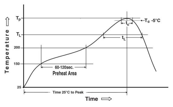
Preheating temperature: 150 ~ 200°C, 60~120 seconds Liquidus temperature (TL): 217°C, 60~150 seconds Peak temperature: 260°C Time within 5 °C of peak temperature (Tc): 255°C, 30seconds
