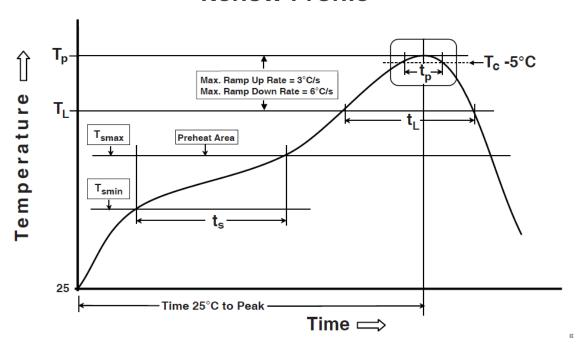
Preheating temperature: 150 ~ 200°C, 60~120 seconds Liquidus temperature (TL): 217°C, 60~150 seconds
