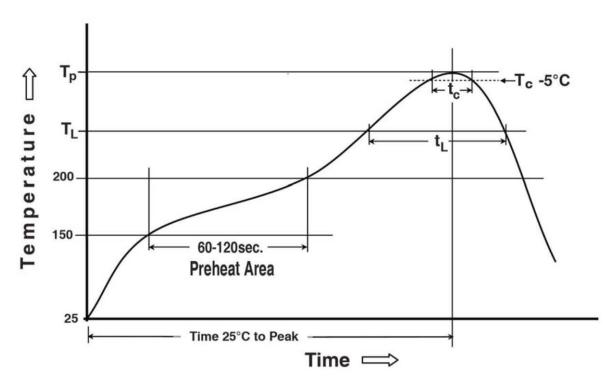
Preheating temperature:  $150 \sim 200^{\circ}$ C,  $60 \sim 120$  seconds Liquidus temperature (TL):  $217^{\circ}$ C,  $60 \sim 150$  seconds
