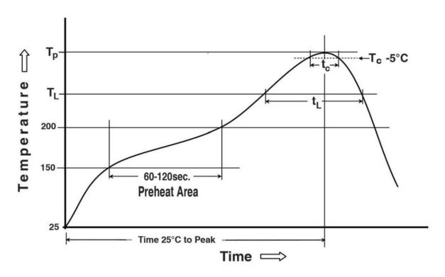
Preheating temperature:  $150 \sim 200^{\circ}\text{C}$ ,  $60 \sim 120$  seconds Liquidus temperature (TL):  $217^{\circ}\text{C}$ ,  $60 \sim 150$  seconds
